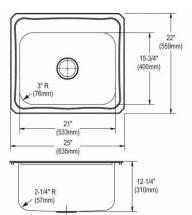
Made in USA Optional Accessories Bottom grid LKWBG2115SS Cutting board CB1516 Drain LK99 Ship dims: 30-11/16" x 26-1/4" x 14" Approx. ship weight: 20 lbs.
