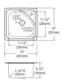
ADA Compliant Made in USA Optional Accessories Bottom grid LKWOBG1111SS Drain LK36 Ship dims: 24-1/4" x 19-3/4" x 9-1/2" Approx. ship weight: 8 lbs.
