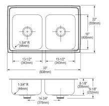
Includes: Two LKPD1 Perfect Drains and strainers. **Built in USA Optional Accessories Bottom grid** LKWBG1316SS **Cutting board** CB1613 CB1713 CBS1316 **Rinsing basket** LKWRB1316SS Drain LKPDVR18B LKDS99 LKDS35 **Ship dims:** 37-3/4" x 26-1/4" x 12-1/2" Approx. ship weight: 29 lbs.
