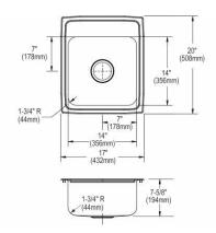
Made in USA Models also available with ADA depths Optional Accessories Bottom grid LKWBG1414SS Cutting board CB1613 Rinsing basket LKWRB1414SS Drain LK99 Ship dims: 21-5/16" x 9-5/16" x 22-15/16" Approx. ship weight: 12 lbs.
