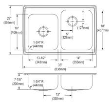
Made in USA **Optional Accessories Bottom grid** LKWBG1316SS **Cutting board** CBS1418 CB1613 CB1713 CBS1316 **Rinsing basket** LKWRB1418SS LKWRB1316SS Drain LK99 Ship dims: 37-3/4" x 26-1/4" x 10-1/2" Approx. ship weight: 21 lbs.
