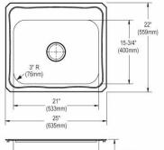
2-1/4\* R (57mm) Made in USA Optional Accessories Bottom grid LKWBG2115SS Cutting board CB1516 Drain LK99 Ship dims: 23-5/16" x 12-1/16" x 31-7/16" Approx. ship weight: 14 lbs.
