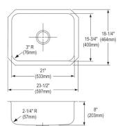
Made in USA Optional Accessories Bottom grid GBG2115SS Cutting board CB1516\* Drain D1125 Ship dims: 23-3/8" x 12" x 31-1/2" Approx. ship weight: 10 lbs. \*1/2" sink reveal required for proper fit.
