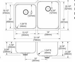
Includes: ELUH3120LPD sink, one LKWOBG1418SS bottom grid, two LKPD1 Perfect Drains and strainers. **Built in USA Optional Accessories Bottom grid** LKWOBG1316SS (small bowl) **Cutting board** CBS1418\* CB1613\* CB1713\* CBS1316\* **Rinsing basket** LKWRB1418SS LKWRB1316SS Drain LKPDVR18B LKDS99 LKDS35 Ship dims: 37-3/4" x 26-1/4" x 14" Approx. ship weight: 32 lbs.
