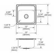
Made in USA **Optional Accessories Bottom grid** LKWBG1209SS **Cutting board** CB912 **Rinsing basket** LKWRB1209SS Drain LK36 Ship dims: 16-5/16" x 9-3/16" x 21-7/16" Approx. ship weight: 7 lbs.
