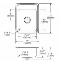
Includes: One LKPD1 Perfect Drain and strainer. **Built in USA Optional Accessories Bottom grid** LKWBG1316SS **Cutting board** CB1613 CB1713 CBS1316 **Rinsing basket** LKWRB1316SS Drain LKPDVR18B LKDS99 LKDS35 Ship dims: 30-11/16" x 26-1/4" x 12-1/2" Approx. ship weight: 18 lbs.
