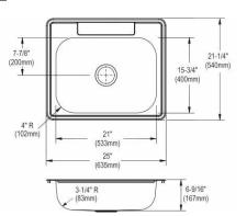
ADA Compliant Made in USA Models also available with ADA depths Optional Accessories Bottom grid GBG2115SS Cutting board CB1516 Drain D1125 Ship dims: 25" x 8-1/8" x 27" Approx. ship weight: 10 lbs.
