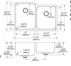
Includes: ELUH3120RPD sink, one LKWOBG1418SS bottom grid, two LKPD1 Perfect Drains and strainers. **Built in USA Optional Accessories** Bottom grid LKWOBG1316SS (small bowl) **Cutting board** CBS1418\* CB1613\* CB1713\* CBS1316\* **Rinsing basket** LKWRB1418SS LKWRB1316SS Drain LKPDVR18B LKDS99 LKDS35 Ship dims: 37-3/4" x 26-1/4" x 14" Approx. ship weight: 31 lbs.
