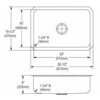
Made in USA Optional Accessories Bottom grid GBG2416SS Drain D1125 Ship dims: 23-5/16" x 9-13/16" x 33-5/16" Approx. ship weight: 23 lbs.
