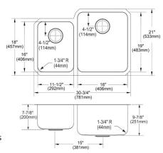
Made in USA Optional Accessories Bottom grid LKWOBG1116SS (small bowl) Rinsing basket LKWRB1418SS (large bowl) LKWRB1116SS (small bowl) \$20 Drain LK99 Ship dims: 37-3/4" x 26-1/4" x 12-1/2" Approx. ship weight: 25 lbs.
