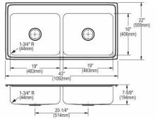
Made in USA Optional Accessories Cutting board CB1713 CBS1316 Rinsing basket LKWRB1418SS Drain LK99 Ship dims: 48-11/16" x 26-1/4" x 10-1/2" Approx. ship weight: 26 lbs.
