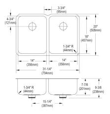
Includes: Two LKPD1 Perfect Drains and strainers. **Built in USA Optional Accessories** Bottom grid LKWOBG1418SS **Cutting board** CBS1418\* **Rinsing basket** LKWRB1418SS Drain I KPDVR18B LKDS99 LKDS35 Ship dims: 37-3/4" x 26-1/4" x 12-1/2" Approx. ship weight: 32 lbs.
