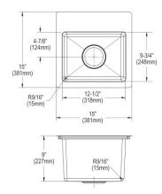
Includes: ECTSR15159T Sink, CTXBG118 Bottom Grid Optional Accessories Drain LKDD LK35 Ship dims: 33" x 24-1/2" x 13" Approx. ship weight: 19 lbs.
