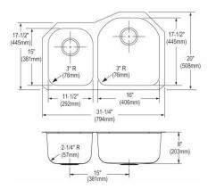
Made in USA Optional Accessories Bottom grid GOBG1617SS (large bowl) GOBG1115SS (small bowl) Drain D1125 Ship dims: 23-5/16" x 9-13/16" x 38-15/16" Approx. ship weight: 19 lbs.
