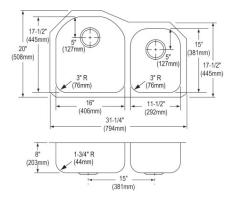
Made in USA Optional Accessories Bottom grid GOBG1617SS (large bowl) GOBG1115SS (small bowl) Cutting board CB1713\* Drain D1125 Ship dims: 21-13/16" x 11-1/16" x 37-3/16" Approx. ship weight: 19 lbs. \*1/2" sink reveal required for proper fit.
