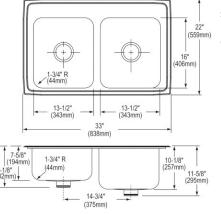
Includes: Two LKPD1 Perfect Drains and strainers. **Built in USA Optional Accessories Bottom grid** LKWBG1316SS **Cutting board** CB1613 CB1713 CBS1316 **Rinsing basket** LKWRB1316SS LKWERBSS Drain LKPDVR18B LKDS99 LKDS35 Ship dims: 37-3/4" x 26-1/4" x 14"
