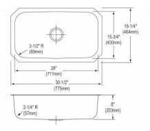
Made in USA Optional Accessories Bottom grid GBG2816SS Drain D1125 Ship dims: 23-5/16" x 9-13/16" x 38-15/16" Approx. ship weight: 16 lbs.
