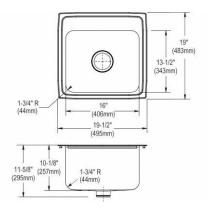
Includes: One LKPD1 Perfect Drain and strainer. **Built in USA Optional Accessories Bottom grid** LKWBG1316SS **Cutting board** CB1613 CB1713 CBS1316 **Rinsing basket** LKWRB1316SS Drain LKPDVR18B LKDS99 LKDS35 **Ship dims:** 26-1/4" x 24-1/4" x 14"
