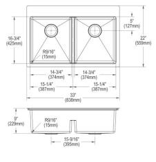
Includes: ECTSRA33229TBG Sink, CTXBG1315 Bottom Grid Optional Accessories Bottom grid CTXBG1315 Drain LKDD LK35 Ship dims: 38" x 24-1/2" x 10-13/16" Approx. ship weight: 34 lbs.
