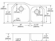
15" (381mm) Includes: ELUH311910R sink, one LKWOBG1617SS bottom grid, one LK99 drain
