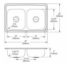
Made in USA Optional Accessories Bottom grid LKWBG1415SS Cutting board CB1516 Rinsing basket LKWERBSS Drain LK99 Ship dims: 23-5/16" x 8-15/16" x 38-15/16" Approx. ship weight: 16 lbs.
