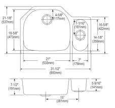
Made in USA **Optional Accessories Bottom grid** LKWOBG2118SS (large bowl) **Cutting board** CB2213 (large bowl) Drain LK99 Ship dims: 37-3/4" x 26-1/4" x 10-1/2" Approx. ship weight: 19 lbs.
