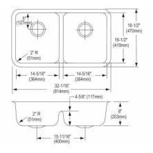
Optional Accessories Bottom grid LKWOBG1416SS Cutting board LKCB1216HW\* Drain LK99 Ship dims: 37-3/4" x 26-1/4" x 10-1/2" Approx. ship weight: 22 lbs.
