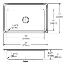
Includes: One LKPD1 Perfect Drain and strainer. **Built in USA Optional Accessories Bottom grid** LKWBG2816SS **Cutting board** CB1713 CBS1316 **Rinsing basket** LKWRB2816SS LKWERBSS Drain LKPDVR18B LKDS99 LKDS35 **Ship dims:** 37-3/4" x 26-1/4" x 12-1/2" Approx. ship weight: 25 lbs.
