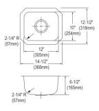
Made in USA **Optional Accessories** Drain D1125 Ship dims: 16-5/16" x 9-3/16" x 19-3/16" Approx. ship weight: 6 lbs.
