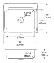
Made in USA Models also available with ADA depths Optional Accessories Bottom grid LKWBG2115SS Cutting board CB1516 Drain LK99 Ship dims: 30-11/16" x 26-1/4" x 10-1/2" Approx. ship weight: 15 lbs.
