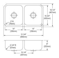
Made in USA Optional Accessories Bottom grid GBG1415SS Cutting board CB1516\* Rinsing basket LKWRB1316SS Drain D1125 Ship dims: 19-9/16" x 11-1/16" x 38-7/16" Approx. ship weight: 17 lbs. \*1/2" sink reveal required for proper fit.
