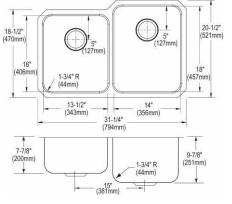
Includes: ELUH3120L sink, one LKWOBG1418SS bottom grid, one LK99 drain **Built in USA Optional Accessories Bottom grid** LKWOBG1316SS **Cutting board** CBS1418\* CB1613\* CB1713\* CBS1316\* **Rinsing basket** LKWRB1418SS LKWRB1316SS Ship dims: 37-3/4" x 26-1/4" x 12-1/2" Approx. ship weight: 27 lbs.
