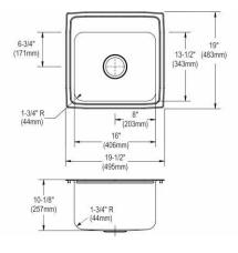
Made in USA Optional Accessories Bottom grid LKWBG1316SS Cutting board CB1613 CB1713 CBS1316 Rinsing basket LKWRB1316SS Drain LK99 Ship dims: 26-1/4" x 24-1/4" x 12-1/2" Approx. ship weight: 14 lbs.
