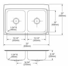
Made in USA Models also available with ADA depths **Optional Accessories Bottom grid** LKWBG1316SS **Cutting board** CB1613 CB1713 CBS1316 **Rinsing basket** LKWRB1316SS Drain I K99 Ship dims: 37-3/4" x 26-1/4" x 10-1/2" Approx. ship weight: 23 lbs.
