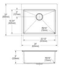
Includes: ECTSR25229T Sink, CTXBG2115 Bottom Grid Optional Accessories Drain LKDD LK35 Ship dims: 33" x 24-1/2" x 13" Approx. ship weight: 24 lbs.
