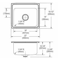
Includes: One LKPD1 Perfect Drain and strainer. Built in USA Optional Accessories Cutting board CBS1418 Rinsing basket LKWRB1418SS Drain LKPDVR18B LKDS99 LKDS35 Ship dims: 30-11/16" x 26-1/4" x 14" Approx. ship weight: 16 lbs.
