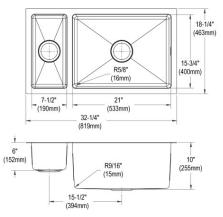
Special Note: Reversible design, sink can be rotated so small bowl is on the left or right Optional Accessories Bottom grid CTXBG1914 CTXBG614 Drain LKDD LK35 Ship dims: 19-15/16" x 12-13/16" x 38-5/8" Approx. ship weight: 40 lbs.
