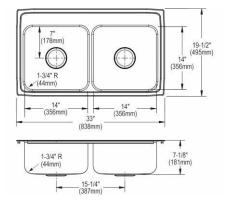
Made in USA Optional Accessories Bottom grid LKWBG1414SS Cutting board CB1613 Rinsing basket LKWRB1414SS Drain LK99 Ship dims: 37-3/4" x 26-1/4" x 10-1/2" Approx. ship weight: 17 lbs.
