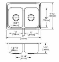
Made in USA **Optional Accessories Rinsing basket** LKWRB1209SS Drain LK99 Ship dims: 23-5/16" x 9-13/16" x 31-3/16" Approx. ship weight: 15 lbs.
