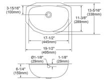
Includes: LKF293 overflow Assembly Built in USA Optional Accessories Drain LK174 LKAD174 Ship dims: 23-5/16" x 19-9/16" x 9-1/16" Approx. ship weight: 8 lbs.
